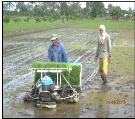
Gambar 20. Alat Tanam Mekanis (Rice Transplanter)
