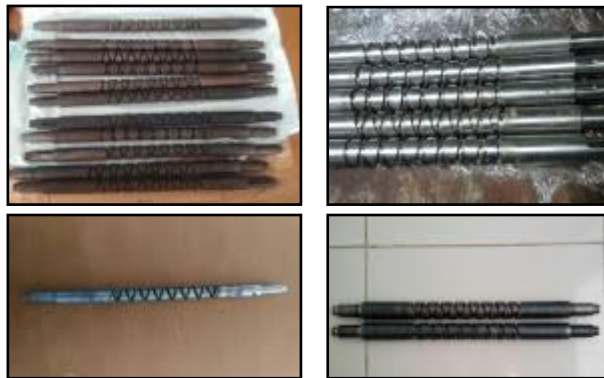
Gambar 12. Standard Manufaktur Self Reversing Screw (Double Screw)
