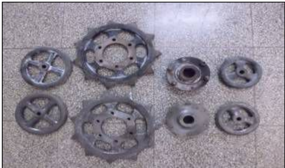
Gambar 16. Komponen-komponen MICO Harvester ( Driving Wheel/Roda Bintang, Roda Penegang Track Shoes )
