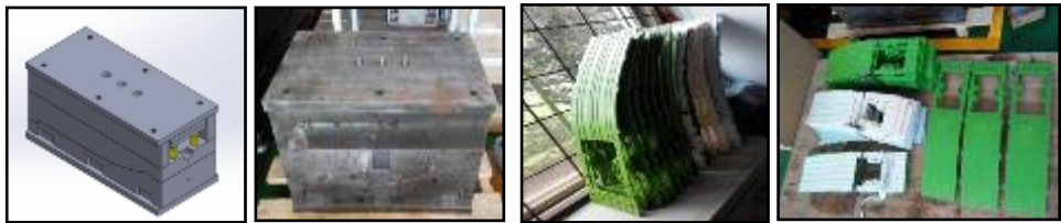
Gambar 9. Mold Prototipe Plastic Injection Papan Bibit (Tray) Indo Jarwo Transplanter (IJT)
